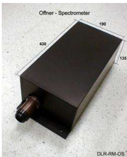
DLR Earth Sensing Imaging Spectrometer (DESI) for integration in the International Space Station's imaging platform for Earth Sensing.
