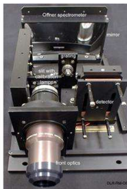
DLR Earth Sensing Imaging Spectrometer (DESI) for integration in the International Space Station's imaging platform for Earth Sensing.
