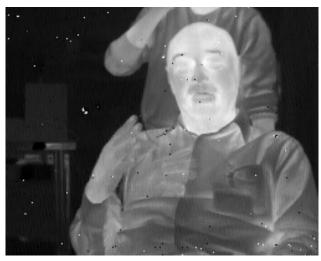
The image shown is not corrected for dead pixels, which is typically done during the image processing in commercial IR cameras.
